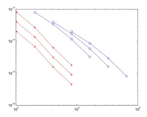
(A2) Error vs. number of micro-steps, stars: SAM with (Strang like) splitting (Kepler+perturbation) micro-integrator 16 macro-steps, circles: standard splitting. Halving  $\epsilon$  halves the error ( $\nu$  = 2).
