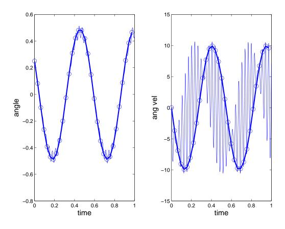
• Stroboscopic samples  $y(t_0)$ ,  $y(t_0+2\pi\epsilon)$ ,  $y(t_0+4\pi\epsilon)$ ,... of y (circles) appear to come from 'smooth' function Y(t). Which Y(t)?
